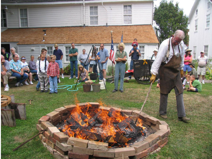
Beth gets a chance to test the tyer for proper temperature (top) before Lonny pronounces it ready for installation (lower)
